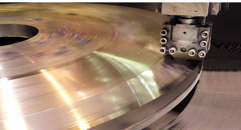
Heavy Duty precision lathe is the largest one for manufacturing molds of oil seals in Taiwan. It completes NAK making molds up the largest diameter 2.3 meters.
